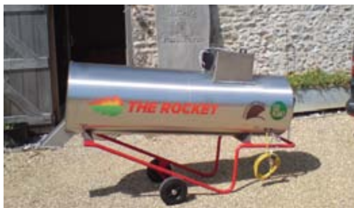
The Rocket in-vessel composter is a relatively state of the art in-vessel composter. When fully operational it produces compost that is pure enough that it can be sold.
